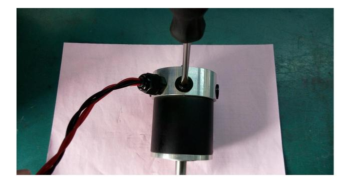
Recommended Brush cap tightening torque levels:
