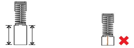
Next, when viewed from the short side, the brush should have a curved cross-section due to continued contact with the commutator. The curve should be centered and not uneven.
