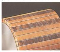
**SLOT BAR MARKING:** Results from a fault in the armature windings. The pattern relates to the number of conductors per slot.
