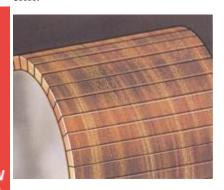
STREAKING: Results from metal transfer to the brush face. Light loads and/or light spring pressure are the most common causes. Contamination can also be a contributing factor.
