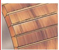
COPPER DRAG: Develops as the commutator surface becomes overheated and softened. Vibration or an abrasive grade causes the copper to be pulled across the slots. Increased spring pressure will reduce commutator temperature.
