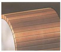
**HEAVY FILM:** Results from high load, light humidity or heavy filming rate grades. Colors not in the brown tones indicate contamination resulting in high friction and high resistance.
