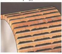
BAR EDGE BURNING: Results from poor commutation. Check 1.) The brush grade has adequate voltage drop, 2.) The brushes are properly set on neutral, and 3.) The interpole strength is correct.
