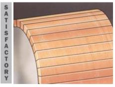
LIGHT FILM: Indicates good brush performance. Light load, low humidity, brush grades with low filming rates, or film reducing contamination can cause lighter color.
