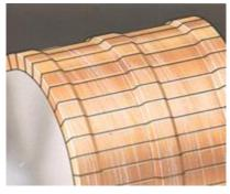
**GROOVING:** May result from an overly abrasive brush grade. The more common cause is poor electrical contact resulting in arcing and the electrical machining of the commutator surface. Increased spring pressure reduces this electrical wear.
