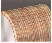
THREADING: Is a further development of the streaking condition as the metal transferred becomes work hardened and machines into the commutator surface. This condition can be avoided by increased loads and increased spring pressure.
