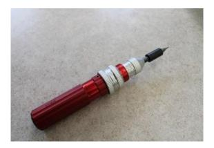
\*It is important to note that the use of the proper sized flat drive bit is essential to success. If a screwdriver or drive bit that is not large enough to fill the entire slot is used the brush cap can easily fail when attempting to remove. This is because all the rotational forces are focused too near the center of the cap and directly at the sharp edges of the driver or drive bit.
